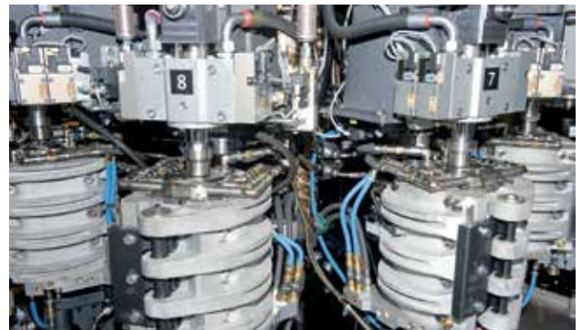
Complete blow mould unit with several moulds/cavities.
