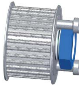
Fig.: 12 Second forcing screw positioned
