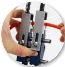
Quick clamp device for inserting the profiles in exchangeable profile jaws.
