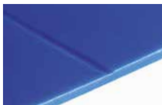
Butt welding with paddle welding tool
